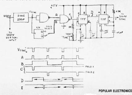
to any line on either field within the range of the circuit. The result is displayed on an oscilloscope. The video signal from a receiver is applied to the vertical input of the scope, while a sync stripper removes the vertical pulse, from which all timing derives. You can extract the vertical pulse from the receiver if desired.
